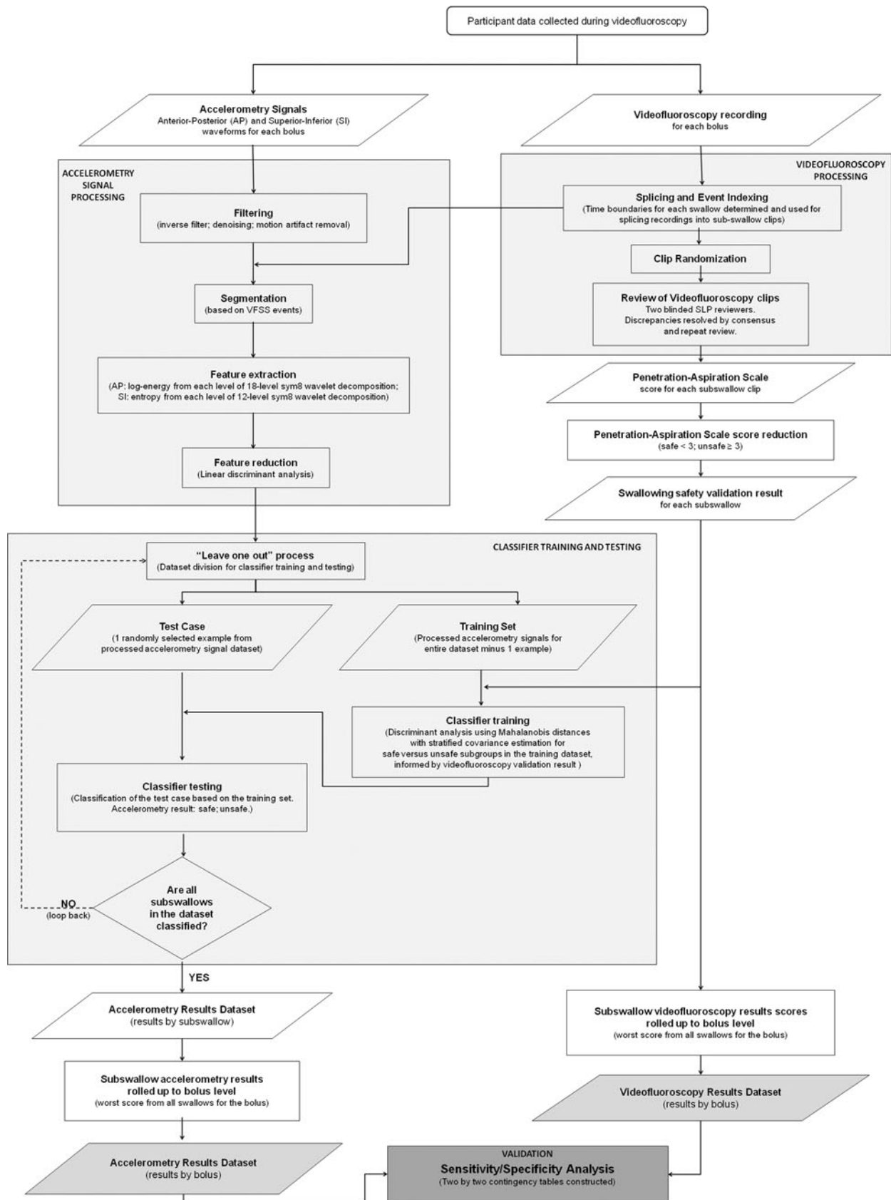
Fig. 2 Flowchart showing the signal-processing steps used to analyze the dual-axis accelerometry signals
